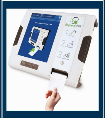
Lee Elections has successfully used the paper-based ExpressVote marking device in every precinct since 2016. The paper-based ExpressVote combines touchscreen ballot marking technology with an integrated thermal printer to produce a paper record for tabulation.
